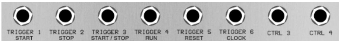
With MIDI Clock selected, the trigger and clock outputs (the first six outputs on the lowest row of the RS370) are reassigned to respond to MIDI Start/Stop/Continue messages as shown in the table at the bottom of this page. To summarise:
